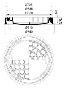
Manhole cover class D 400 for individual surface, round, without ventilation, frame height: 100 mm, with damping insert MEIPREN®
