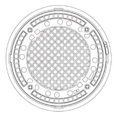
Manhole cover class C 250, round, surface water-proof, with 4 lockings and oil- and petrol resistant sealing, frame height 70 mm
