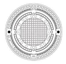
Manhole cover class D 400, self-levelling, System MEILEVEL®-A, round, without ventilation, with rounded frame (especially for use in areas with snowploughs), frame height 160 mm
