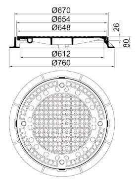
Manhole cover class A 15, test force 50 kN, round, without ventilation, frame height 80 mm
