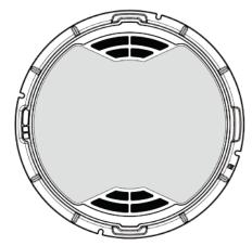
Manhole cover class C 250, round, with ventilation, frame height 80 mm
