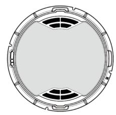
Manhole cover class B 125, round, with ventilation, frame height 80 mm
