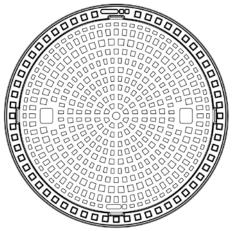
Manhole cover class B 125, round, without ventilation, frame height 125 mm
