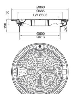
Manhole cover class D 400 self-levelling, System MEITOP®-S, round, without ventilation, with safety hinge and 2 spring locks, incl. damping insert in the frame, for use with adjustment rings conform DIN 4034, frame height 190 mm
