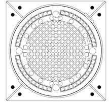
Manhole cover class F 900 square, without ventilation, frame height 100 mm
