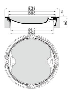
Manhole cover class D 400 round, without ventilation, frame height 160 mm with damping insert MEIPREN®
