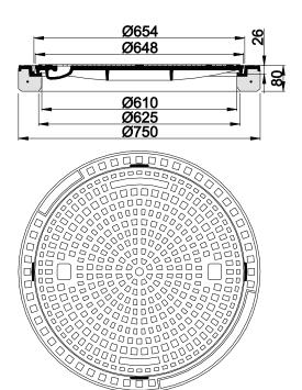
Manhole cover class A 15, test force 50 kN, round, without ventilation, incl. sand-seal frame height 80 mm
