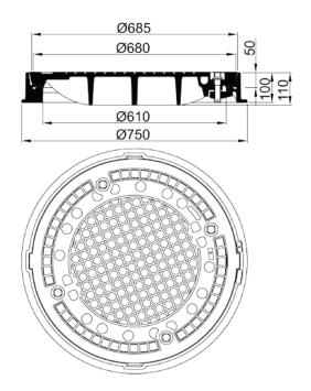
Manhole cover class D 400 round, surface water-proof, with 4 lockings and oil- and petrol resistant sealing, frame height 100 mm
