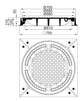
Manhole cover class E 600 square, without ventilation, with damping insert MEIPREN® in cover, frame height 100 mm
