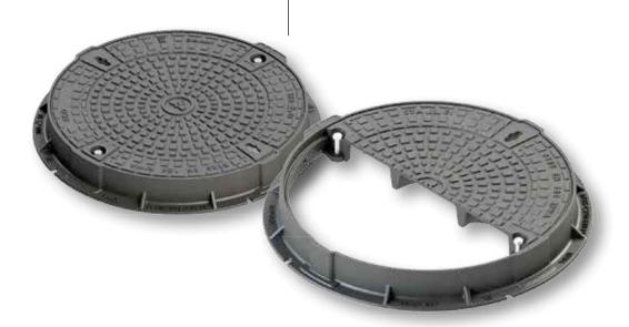
Manhole covers with safety locking devices are secured against unauthorised opening, and lifting due to backpressure, using a catch which swivels into a frame recess and is then firmly tightened. A force-fitting connection is therefore provided. Manhole covers with locking devices are always supplied without damping inserts for safety reasons.
