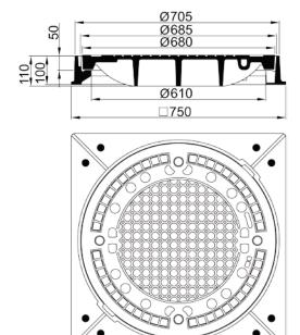
Manhole cover class D 400 square, without ventilation, frame height 100 mm
