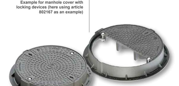
Manhole covers with safety locking devices are secured against unauthorised opening, and lifting due to backpressure, using a catch which swivels into a frame recess and is then firmly tightened. A force-fitting connection is therefore provided. Manhole covers with locking devices are always supplied without damping inserts for safety reasons.
