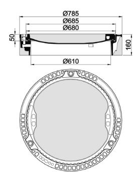
Manhole cover class D 400 round, surface water-proof up to 0.5 bar, with 3 screw connections and oiland petrol resistant sealing, frame height 100 mm
