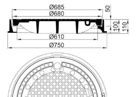
Manhole cover class E 600 round, without ventilation, frame height 100 mm
