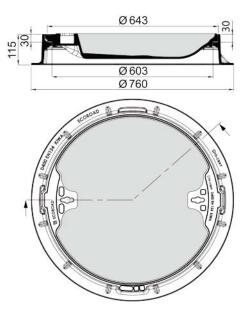
Manhole cover class D 400 System ECOROAD® round, without ventilation, frame height 115 mm
